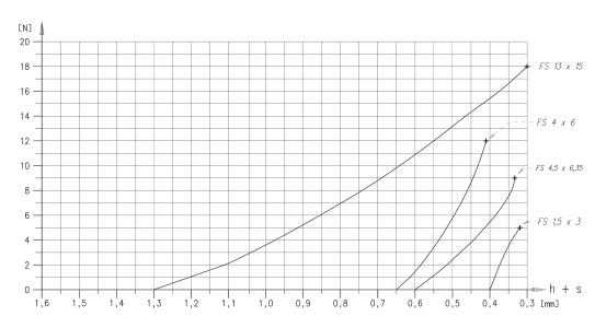
h+s at F=0N measured with 0.36N Characteristic curves apply to not set precision spring washers
