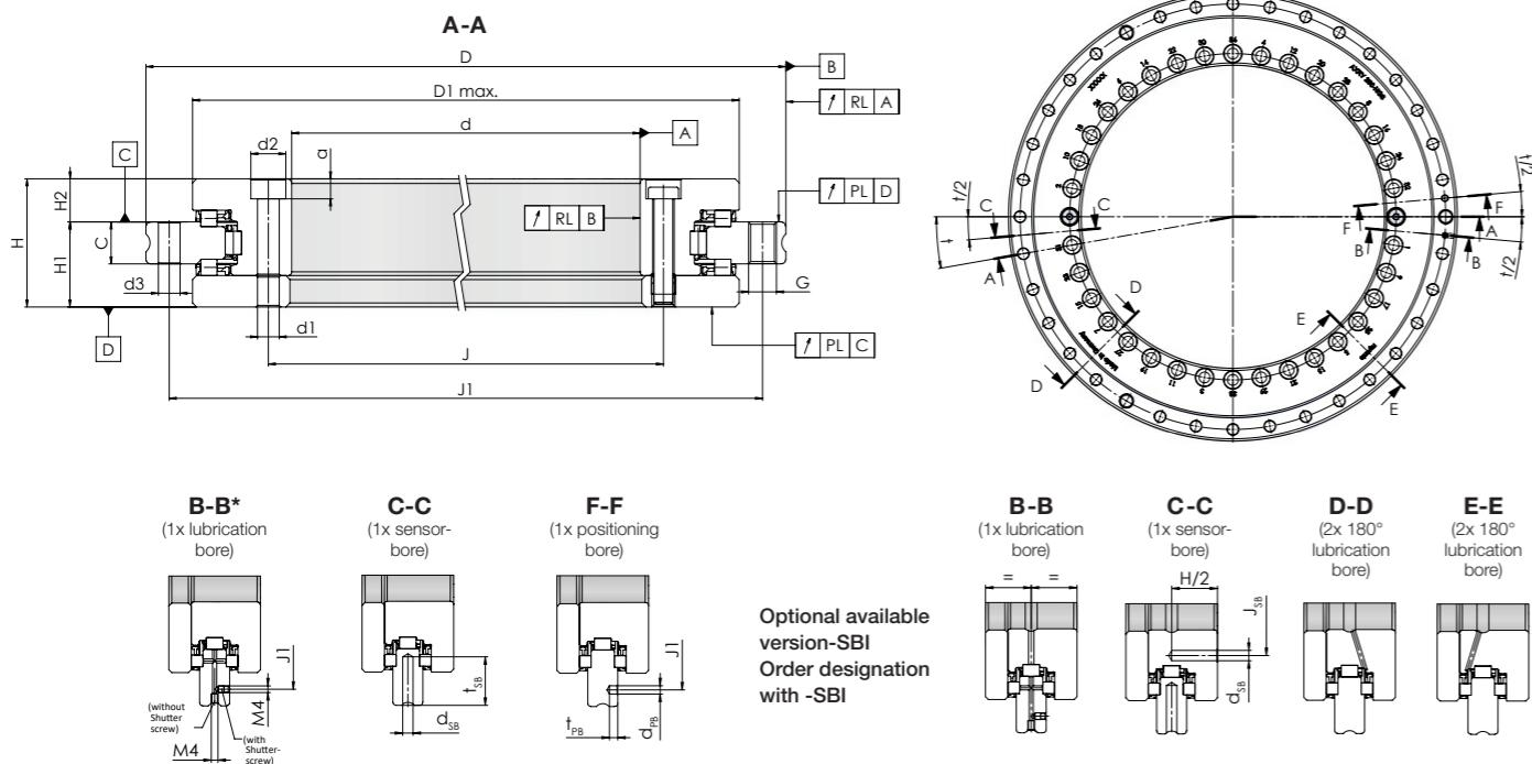
\*Note: In the case of axial lubrication, please remove the screw plug and seal off the radial lubrication!
